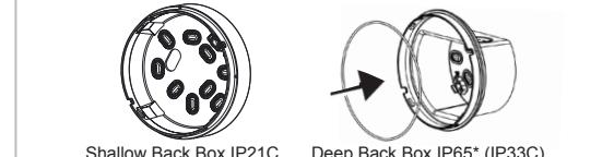
**(ENG)** If the Deep IP65 option is used, the O-ring seal must be fitted as shown. If required, the deep back box gasket accessory can be installed between the back box and the mounting surface. \*IP33C is certified by LPCB to EN54-3 and EN54-23. IP65 is certified by UKAS Accredited test facility.
