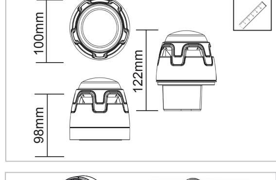
**(ENG)** If the Deep IP65 option is used, the O-ring seal must be fitted as shown. If required, the deep back box gasket accessory can be installed between the back box and the mounting surface. IP33C is certified by LPCB to EN54-3 and EN54-23. IP65 is certified by UKAS Accredited test facility.
