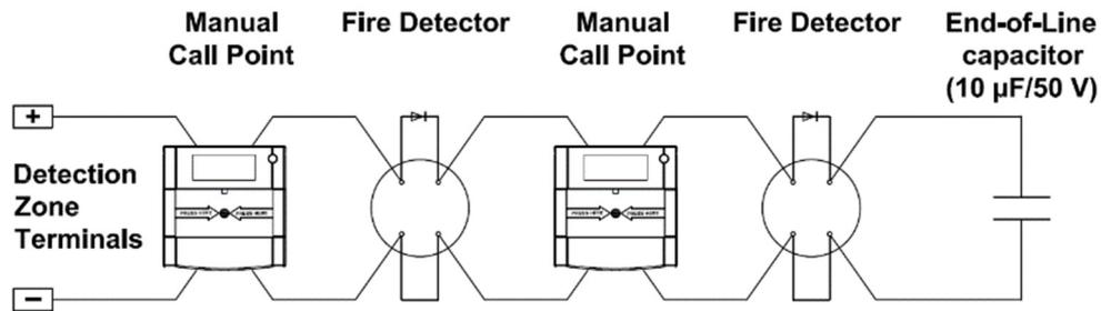
If manual call points are wired on the same circuit as detectors, then in order to comply with some local requirements regarding device disconnection monitoring, detector bases should have a Schottky diode fitted which permits manual call points to continue to operate normally after a detector is removed (see diagram). Manual call points should have a maximum internal resistance of (470 ~ 680) Ω when activated.
