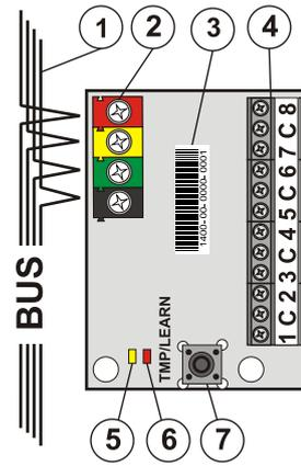
Fig 2: 1 – BUS cable; 2 – BUS terminals; 3 – production code (on the bottom of the PCB); 4 – input terminals for external magnetic detectors; 5 – yellow LED; 6 – red LED; 7 – tamper contact
