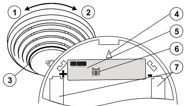
Fig 6: 1– opening the detector cover; 2 – closing the detector cover; 3 – optical status indication; 4 – arrow showing where to insert the detector; 5 – production code; 6 – external antenna connector; 7 – battery holders;
