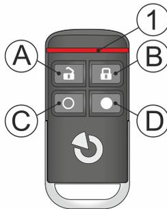
Figure: 1 – LED indication A, B, C, D – buttons, see their functions according to table 1.
